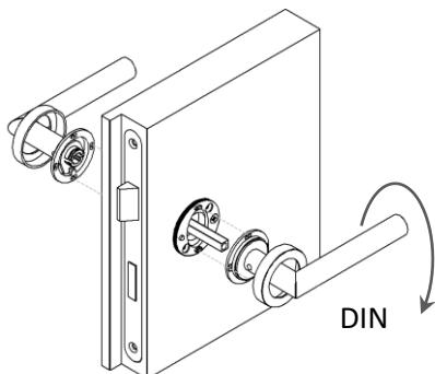
Place the lever base rose on the spindle and push onto the mounting plates. Pay attention to the direction of the lever handles ensuring they can be pressed downwards.
