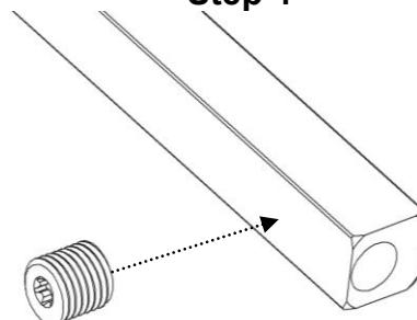
**Attention:** Insert the spindle in such a way that the point of the grub screw can break through the thinnest side.
