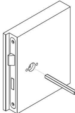
Drill a 19mm hole in the door to allow the spindle to be located through the lock follower.
