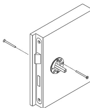
Fix the rose mounting plates (metal) and secure with the M4 bolt through fixings.
