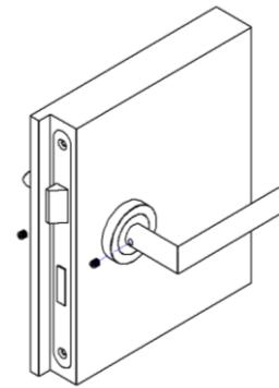
Tighten the grub screws on both levers ensuring they pierce the spindle.
